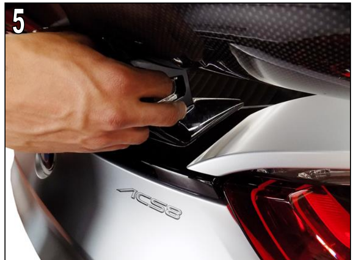
Fig. 4 – 6 Place the AC Schnitzer rear wing on the vehicle and align.
