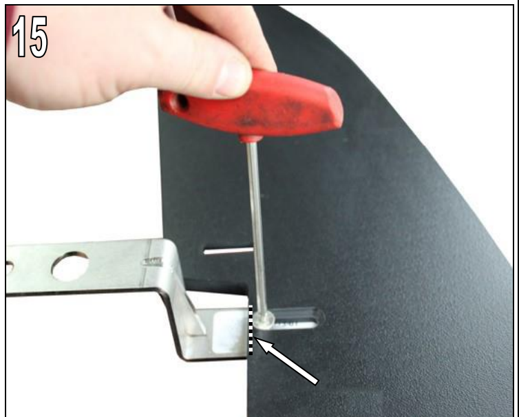
Fig. 15 Mount the AC Schnitzer fixing bracket to the AC Schnitzer front splitter using the countersunk head bolt M6x10mm supplied, and tighten.
