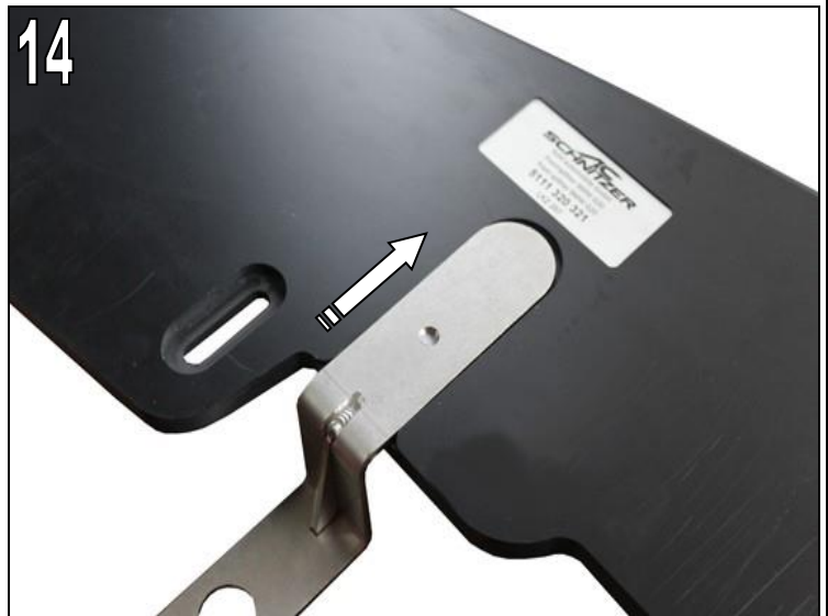
Fig. 14 Lay AC Schnitzer fixing bracket in the AC Schnitzer front splitter as shown.
